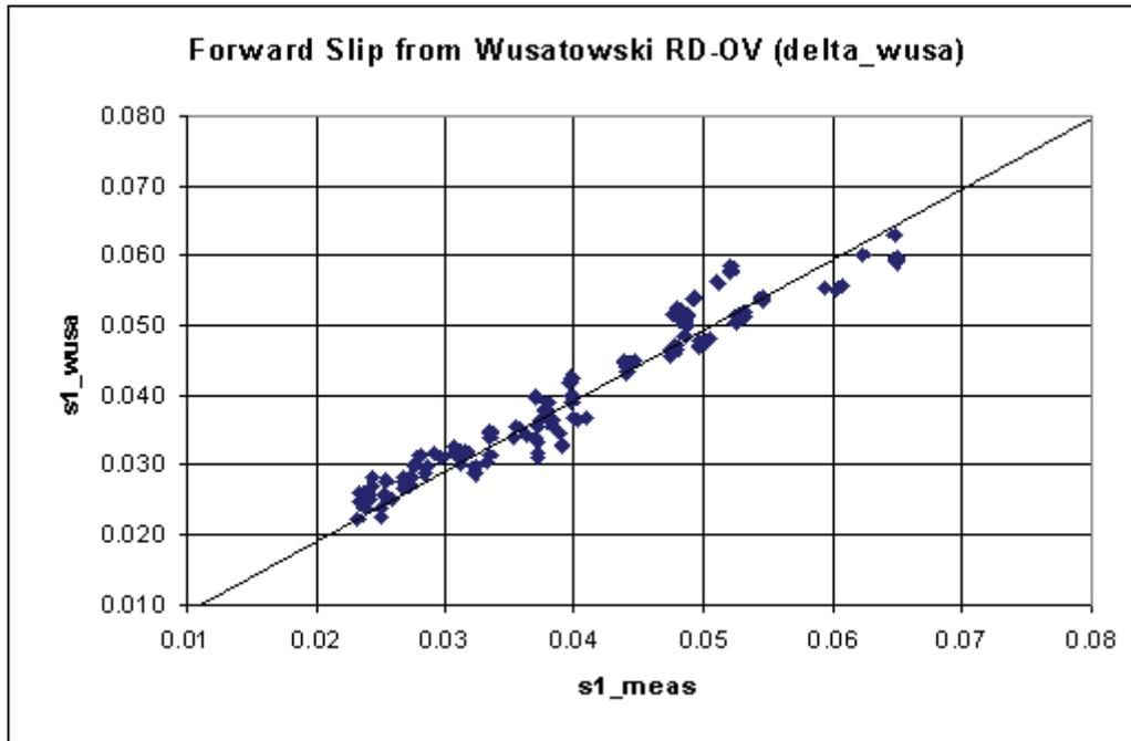
Fig. 3: Predicted forward slips and measured values in the lab mill data (based on Wusatowski and a new model for neutral angle)
