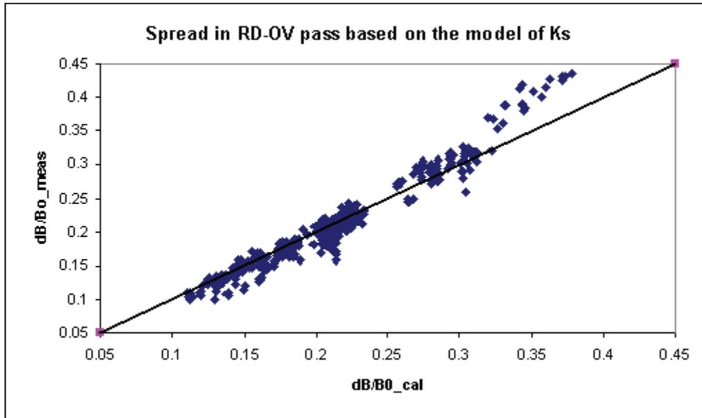
Fig. 1: Calculated  $\Delta B/B_0$  values for RD-OV with modified Shinokura, in comparison with the measured ones
