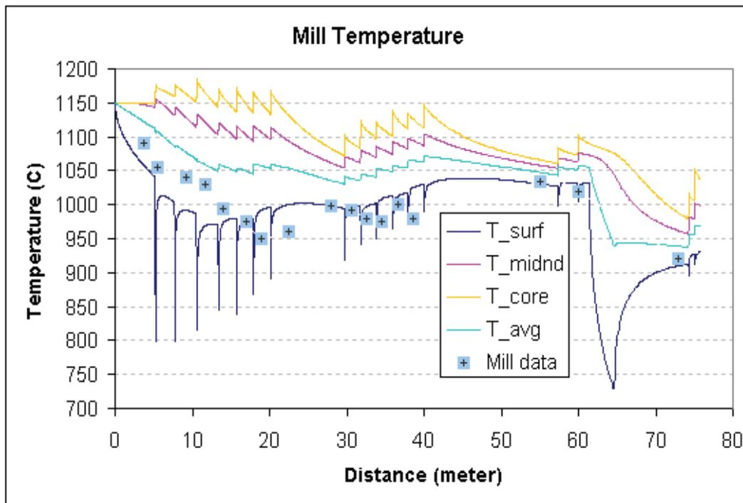
Fig. 5: Calculated temperature profile with comparison with the measured surface temperature
