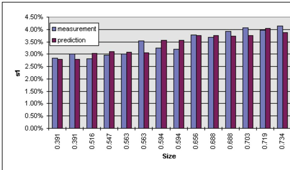
Fig. 4: Predicted forward slips and measured ones in the finish passes of a production rolling block (size in inch)
