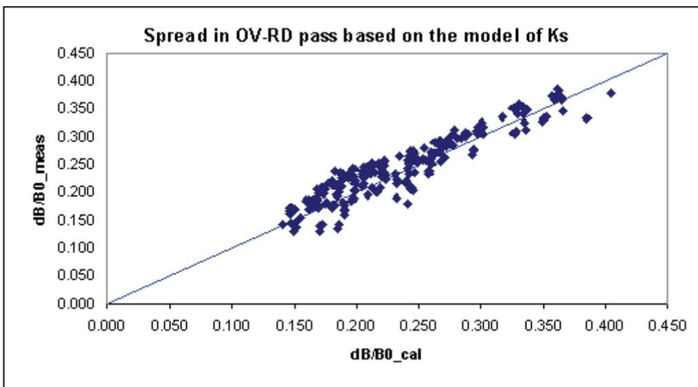
Fig. 2: Calculated  $\Delta B/B_0$  values for OV-RD with modified Shinokura, in comparison with the measured ones
